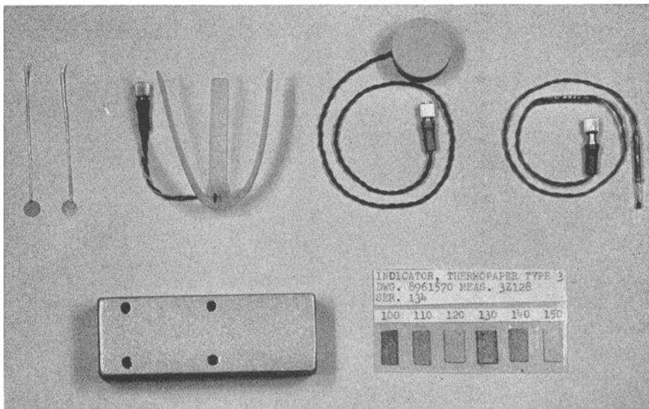
Fig. 6. Transducer assemblies for Bio-Flight 1. The top row shows the two electrocardiogram electrodes, the respiration rate transducer mounting, the chest sound microphone, and the body temperature thermistor. A nuclear track plate package and a flash temperature indicator card are shown in the bottom row.
