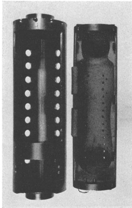
Fig. 3. Basic animal support cylinders for Bio-Flight 1. The cylinder on the right contains the ventilated, contoured support bed and is fitted into the outer protective cylinder on the left. Ventilation holes are shown clearly.
