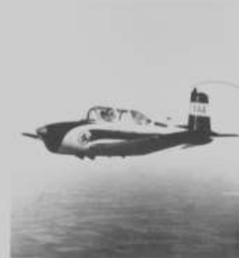
The T-34 Beechcraft in flight. The flying laboratory, only one of its kind, uses 30 radio channels to send information to the ground recorder.
