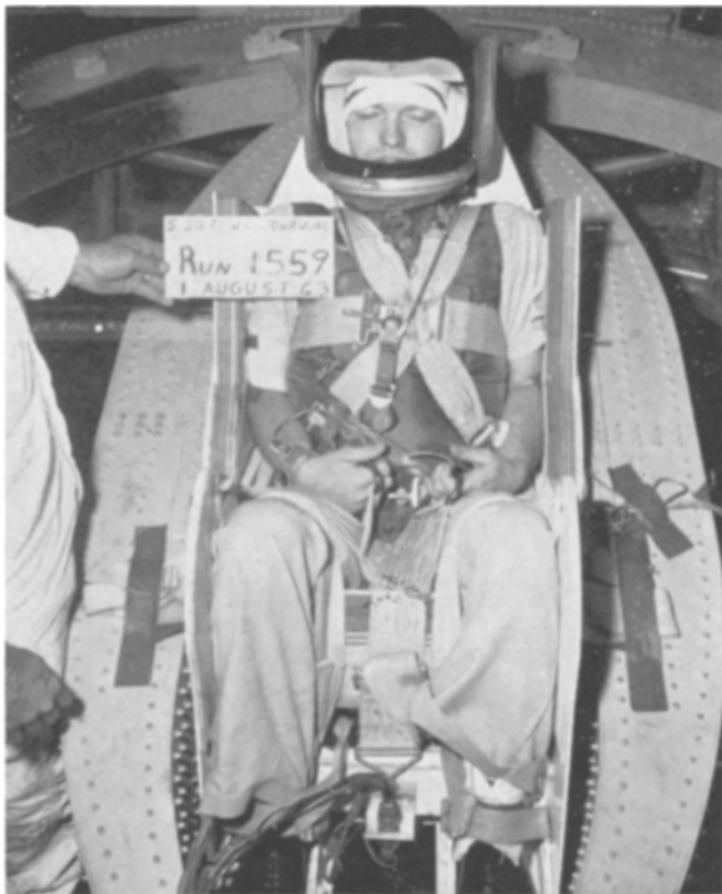
Fig. 3. Helmet and Restraints. Subject in firing position, wearing Mercury helmet attached to neck ring on Nylon vest, anchored to strap passing under the crotch. Apollo Dacron webbing restraint harness with shoulder straps, chest belt, seat belt, thigh straps, ankle straps and hand holds. Between feet and at right, instrumentation leads to trailing cable.
