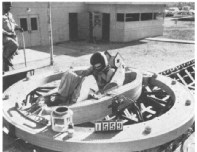
Fig. 2. Omni-directional sled. Horizontal ring, 3.05 meters in diameter, with bolt holes for 10° increments of yaw positioning of cradle, suspended between gimbals providing for 10° increments of positioning in roll; contained between gimbals in the cradle is the seat, locked in pitch position 45°, tipped back from vertical, or 0° pitch. Trailing cable in lower right corner of picture links sled instrumentation to recording station in upper right.
