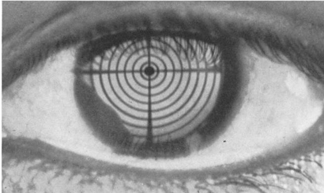
Fig. 5. Placido disk reflection on cornea at 1 g.
