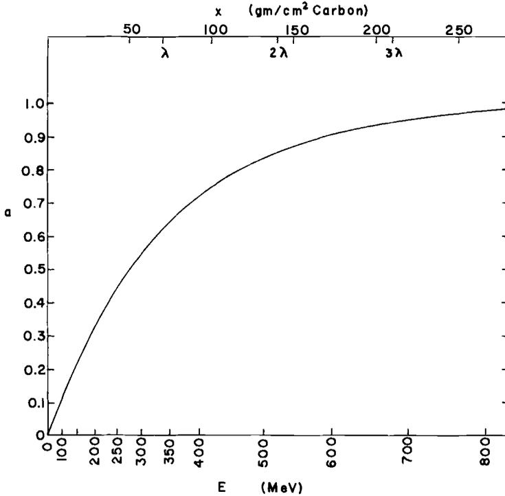
Fig. 1. Fraction *a* of incident protons undergoing nuclear interaction in a carbon shield vs. the path length *x* traversed in carbon (upper abscissa). The lower abscissa gives the energy *E* of a proton whose range is as given in the upper abscissa. The mean free path  $\lambda$  for (inelastic) nuclear interaction in carbon is about 70 gm/cm<sup>2</sup>.
