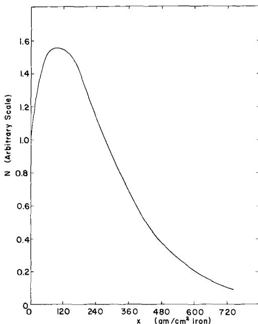
Fig. 3. Calculated flux of the nuclear-interacting component  $N$  vs. depth  $x$  in iron. Incident spectrum: normal non-solar cosmic rays. Calculations based on Martin's model. (This graph is not intended to be used for estimating actual shield thicknesses).
