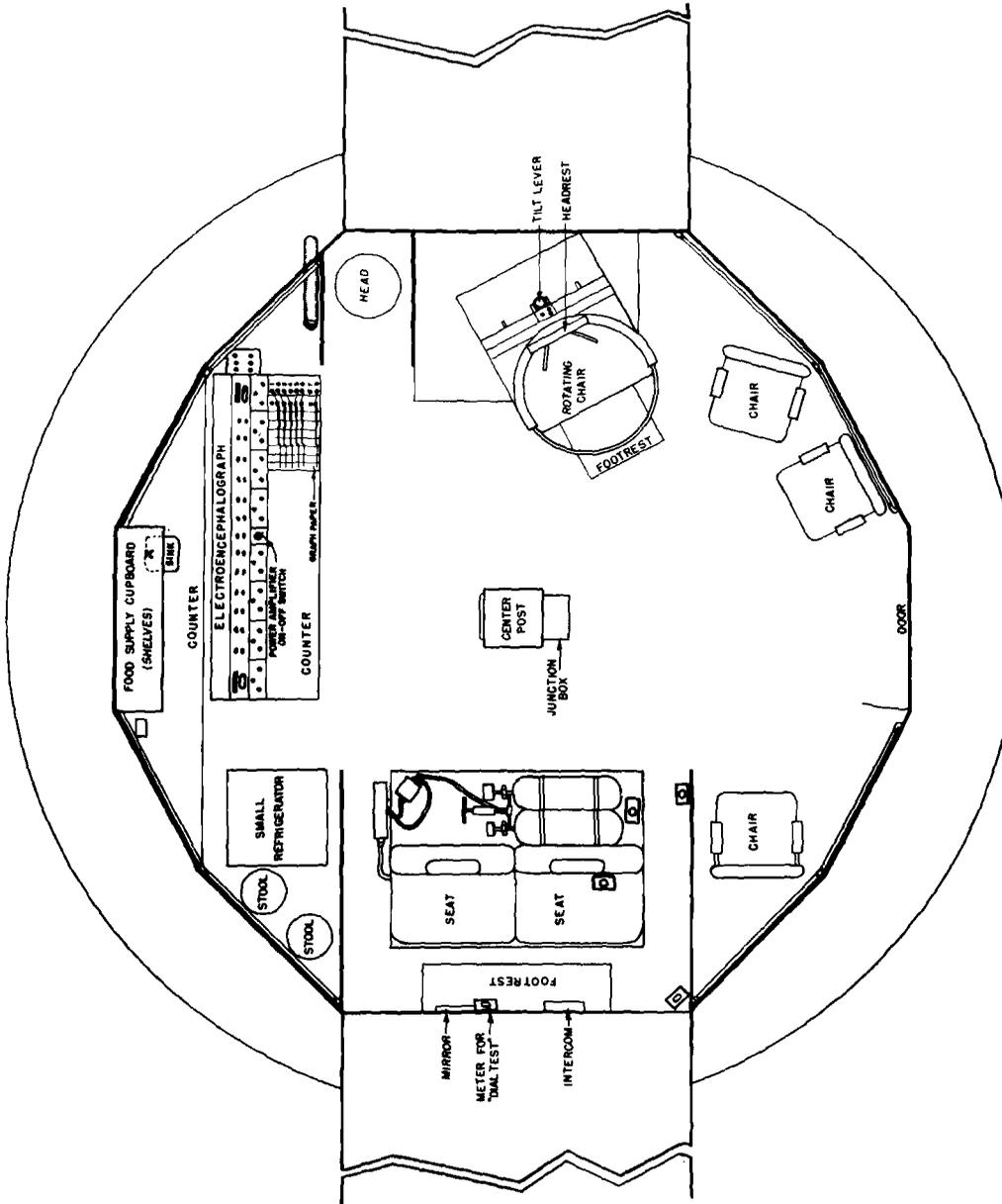
Fig. 1. Floor plan of Pensacola Slow Rotation Room.
