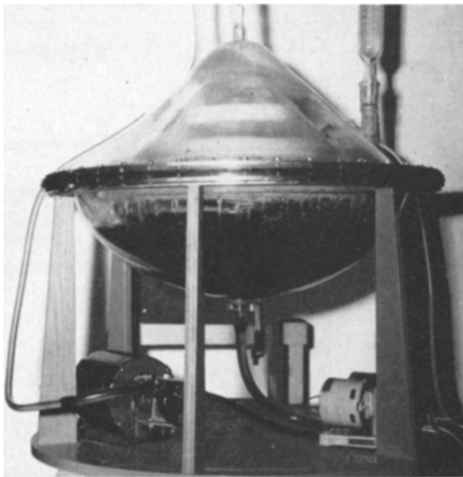
Fig. 5. Algal photosynthetic gas exchanger basically composed of two parts. The algae are collected in a hemispheric container and continuously recycled over a conical illuminated surface.
