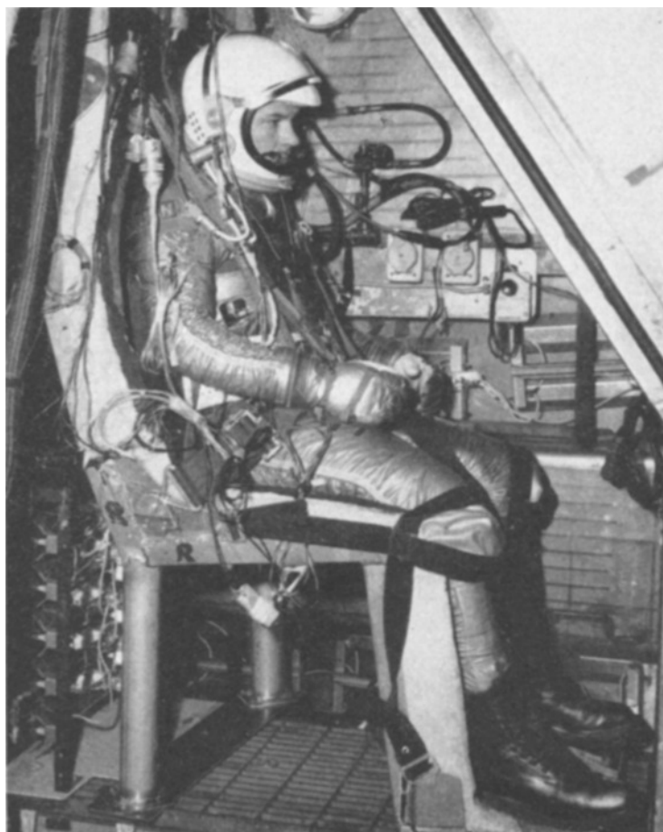
Fig. 1. Subject wearing full pressure suit while seated in thermal test chamber.
