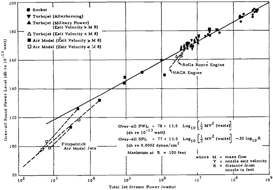
Fig. 1. The over-all acoustic power of engines.
