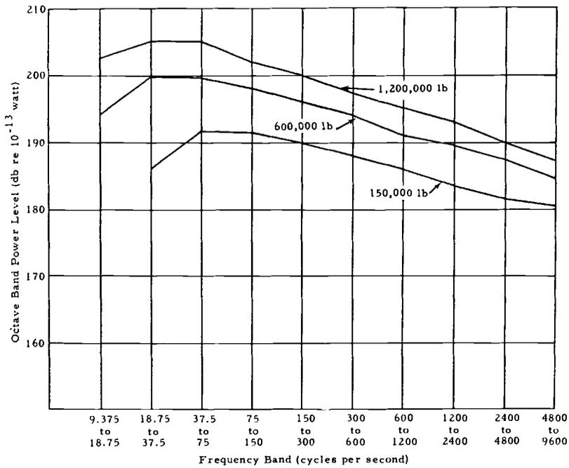
Fig. 2. Predicted acoustic power level spectrum for three large rockets.
