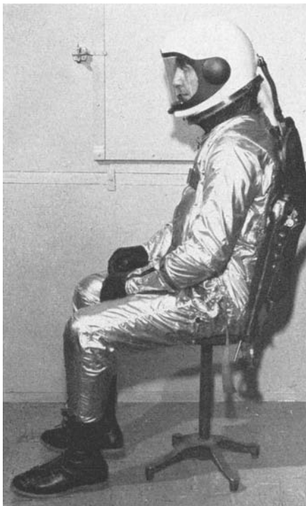
Fig. 1. The MC-2 full pressure suit.
