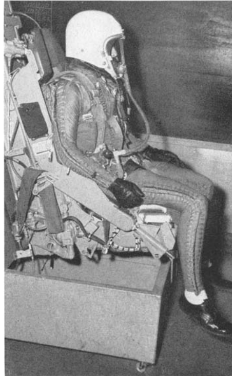
Fig. 2. The subject is wearing the MC-4 partial pressure suit, MA-2 helmet, and parachute, and is seated in an ejection seat.
