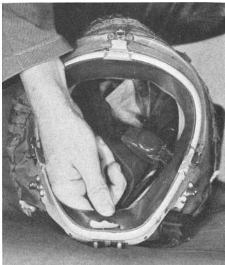
Fig. 3. Tear in rubber face seal in MA-2 helmet (Case 2).
