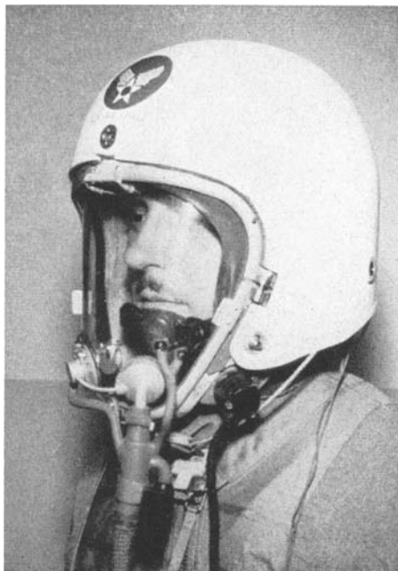
Fig. 4. The subject is wearing the MA-2 helmet incorrectly with rubber gasket on outside of face mask.
