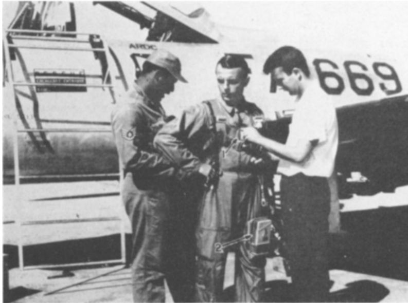
Fig. 5. Pre-flight preparation of subject. On the chest belt (1) is a sensitive accelerometer for recording G values near the zero mark, and (2) on left leg is miniaturized tape recorder to assure preservation of verbal data in case of radio or ground-station recording failure.
