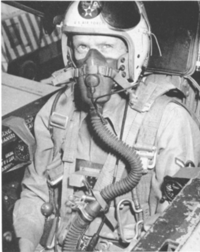
Fig. 4. Subject in cockpit, showing mounting of clock (at left upper arm) and accelerometer (right) for use in analysis of motion pictures.
