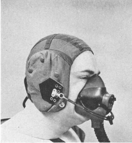
Fig. 3. Subject pressure breathing at 52 mm. Hg. with RAF type "N" pressure breathing mask and toggle harness.
