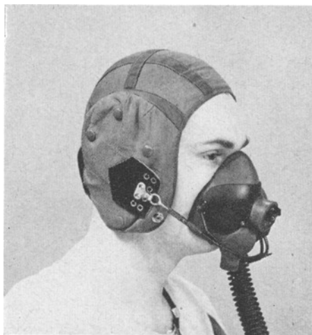
Fig. 2. Subject wearing RAF Type "N" pressure breathing mask with toggle harness.
