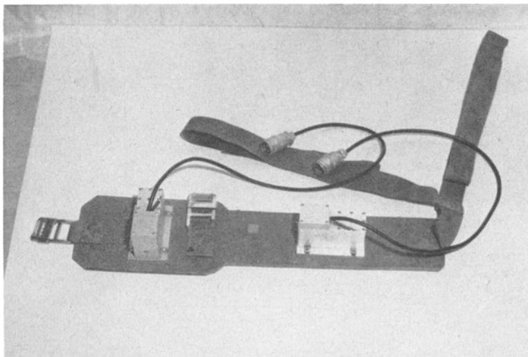
Fig. 3. Statham accelerometers mounted on chest band for recording quantitatively G forces on subjects during sub-gravity trajectory. Accelerometer at left is oriented to record longitudinal G forces, and at right, vertical forces.
