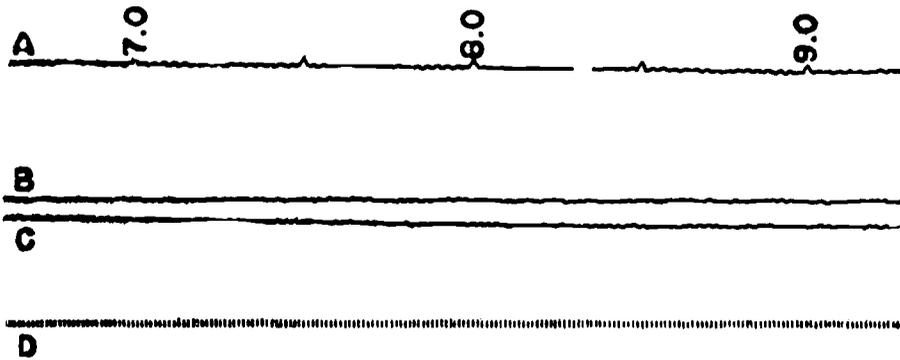
Fig. 5. A segment of oscillograph record of sub-gravity flight, showing: (A) timing in seconds, (B) vertical G force, (C) longitudinal G force, and (D) 100 cps timing tracing.
