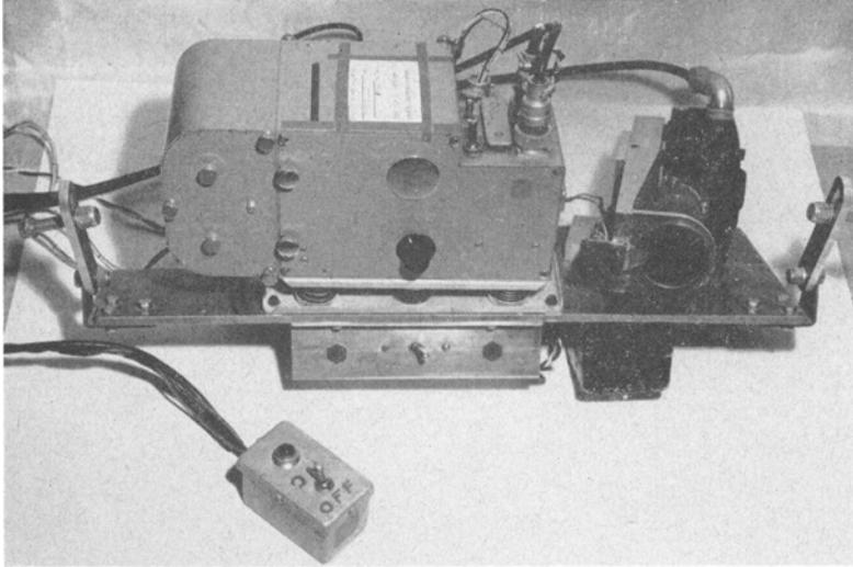
Fig. 4. Century model 409 oscillograph recorder and gun sight aiming point gun camera with 84° wide angle lens.
