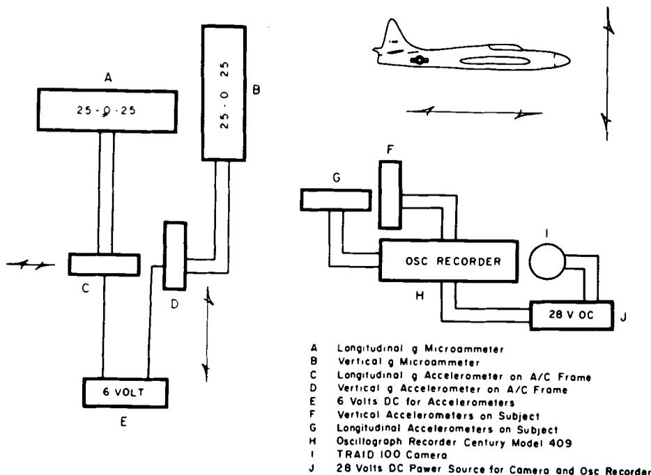
Fig. 6. Block diagram of instrumentation used in sub-gravity tests.
