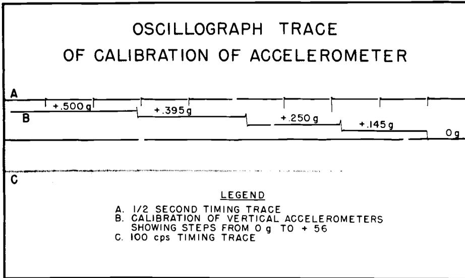
Fig. 7. Oscillographic tracing of calibration of accelerometer, showing: (A) timing in 1/2 second units; (B) steps in vertical accelerometer from zero G to +0.56 G, and (C) 100 cps timing tracing.
