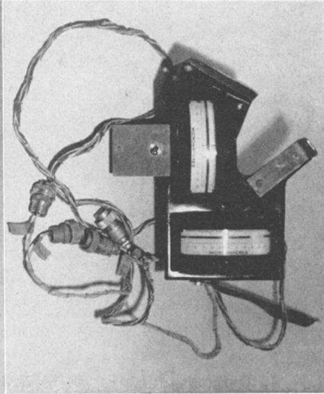
Fig. 2. Microammeters with range of 25-0-25 microamperes and bracket for installation in pilot's compartment of F-94 type aircraft.
