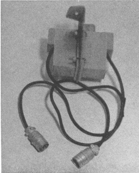
Fig. 1. Statham  $\pm 0.5$  G accelerometer and bracket used for mounting on aircraft frame.
