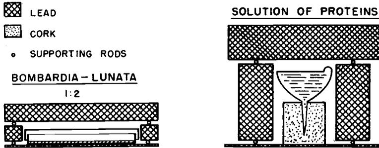
Fig. 6. Cosmic ray shower experiment. Optimal lead shielding 15 mm. (After Rajewsky, Krebs and Zickler, and Rajewsky, Krebs and Kasten.)
