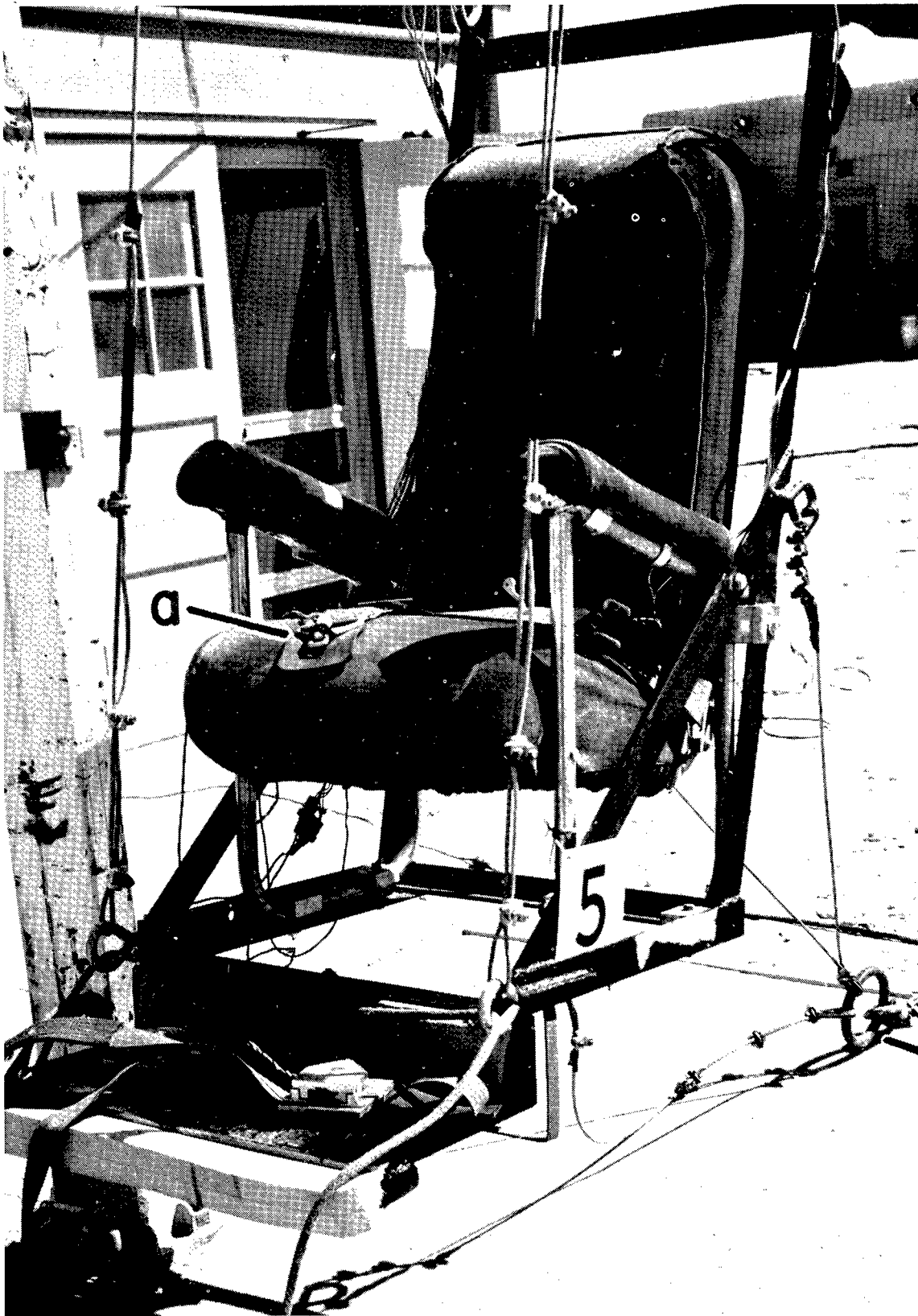
Swing Seat with a. Three-Inch-Wide Lap Belt b. Snub Cable Decelerator
