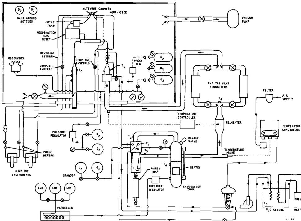
Fig. 1. Schematic diagram of environmental control system used in this experiment.
