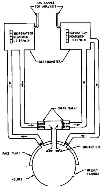
Fig. 2. Schematic diagram of respiratory circuit.
