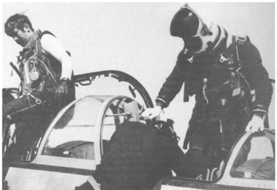
EMERGENCY PRESSURE JERKIN —Canadian pilots have successfully tested a lightweight jerkin with an inflatable bladder for use in emergency decompression. In a test to 60,000 ft., the jerkin—a sleeveless vest—allowed positive pressure breathing above the ambient pressure until a safe altitude was reached. Leaving a CF 104 Starfighter after the test is test pilot Capt. John MacNamara, left, wearing the jerkin, and safety pilot Capt. Jerry Nicks, wearing a full pressure suit.
