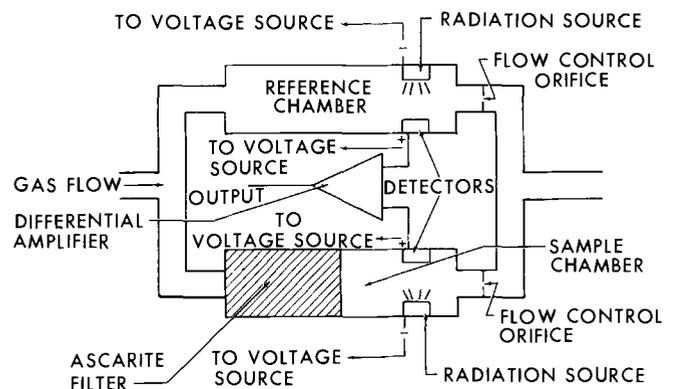
Fig. 5. Radiation Absorption System.
