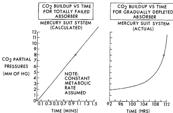
Fig. 1. Typical CO<sub>2</sub> Buildup Rates for Failed LiOH Canister.
