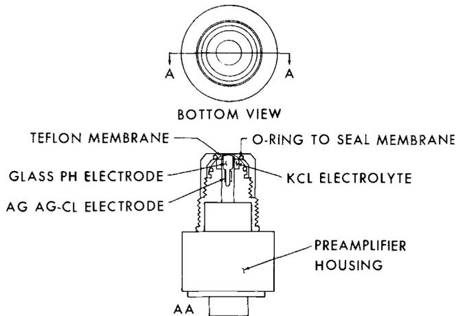
Fig. 3. Mercury CO<sub>2</sub> Measuring System Sensor Portion.
