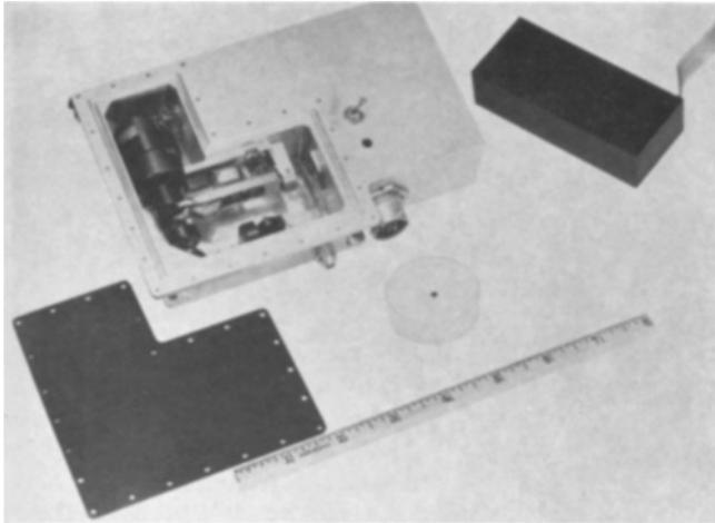
Fig. 6. Apollo CO<sub>2</sub> Measuring System.
