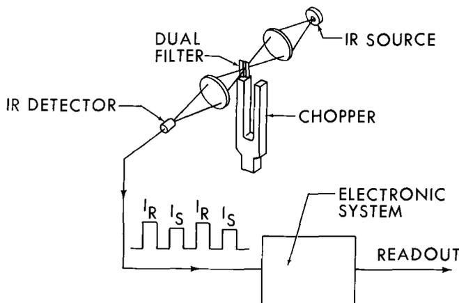
Fig. 7. Infrared CO<sub>2</sub> Sensor.
