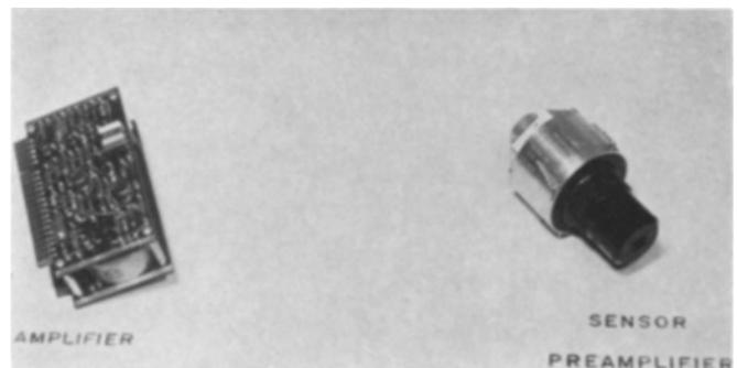
Fig. 2. Mercury CO<sub>2</sub> Sensing System.
