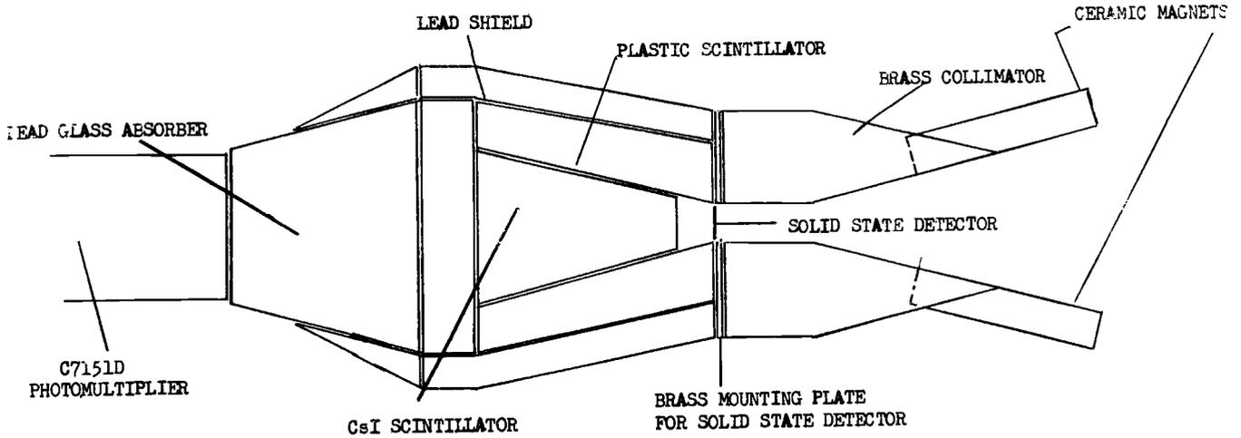
Fig. 1. Charged particle and gamma detector.
