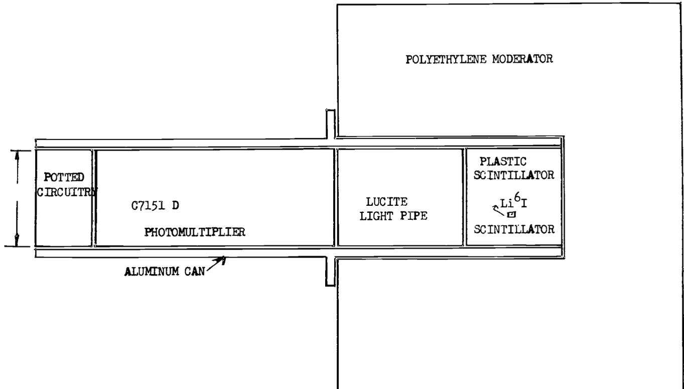
Fig. 2. Neutron detector.
