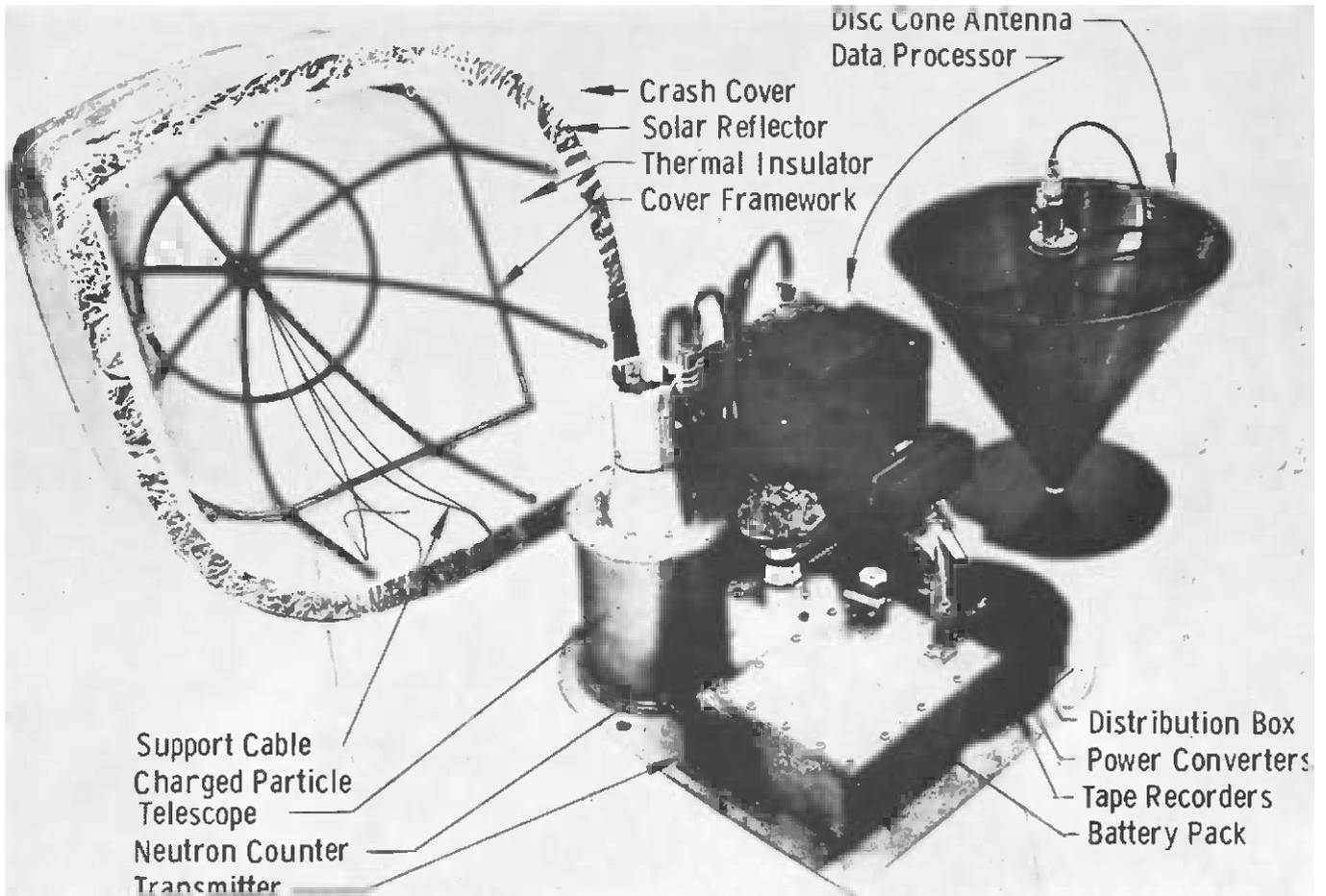
Fig. 4. Space radiation monitoring system, equipment.
