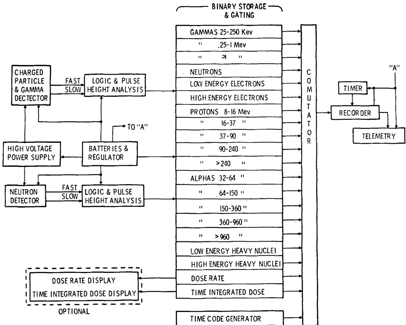
Fig. 3. Space radiation monitoring system functional block diagram.
