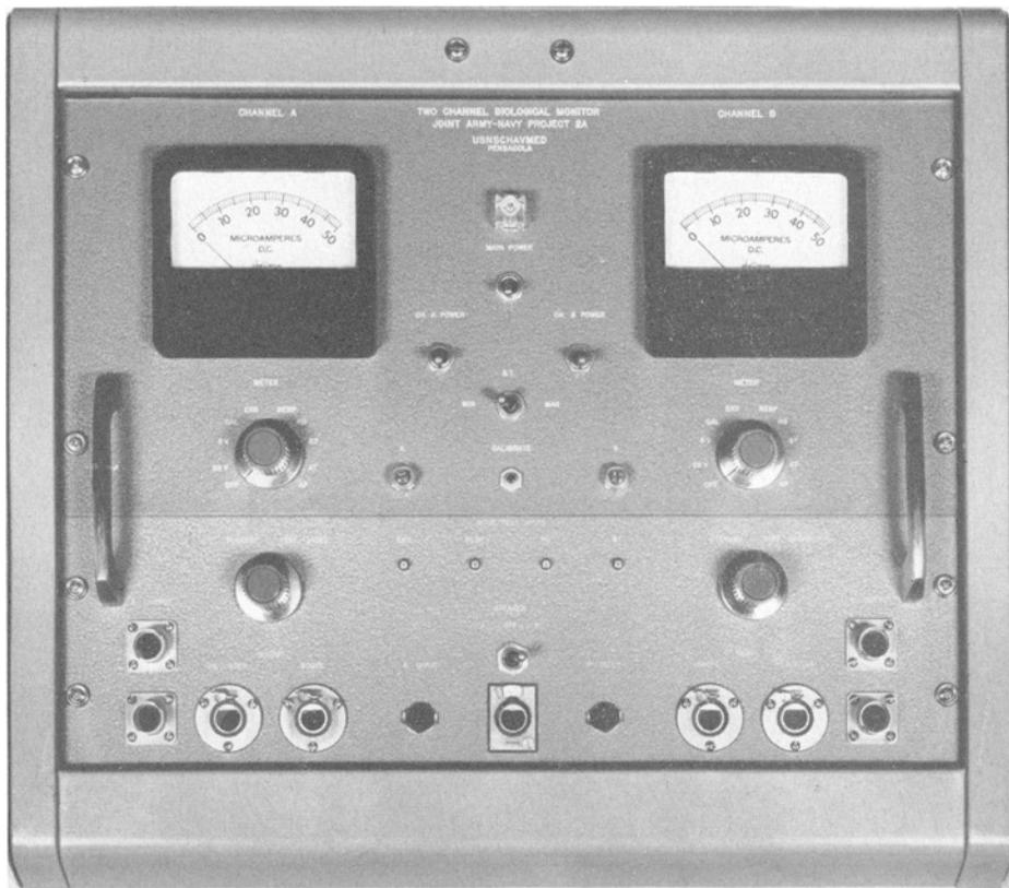
Fig. 20. Front view of biological monitor for Bio-Flight 2 Baker electronic system.
