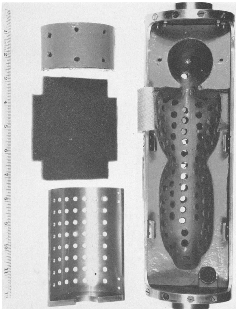
Fig. 18. Components of animal support assembly for Bio-Flight 2 Baker. The cylinder with ventilated contour bed is shown on the right. On the left from top to bottom; chest pad, cover plate liner and cover plate.
