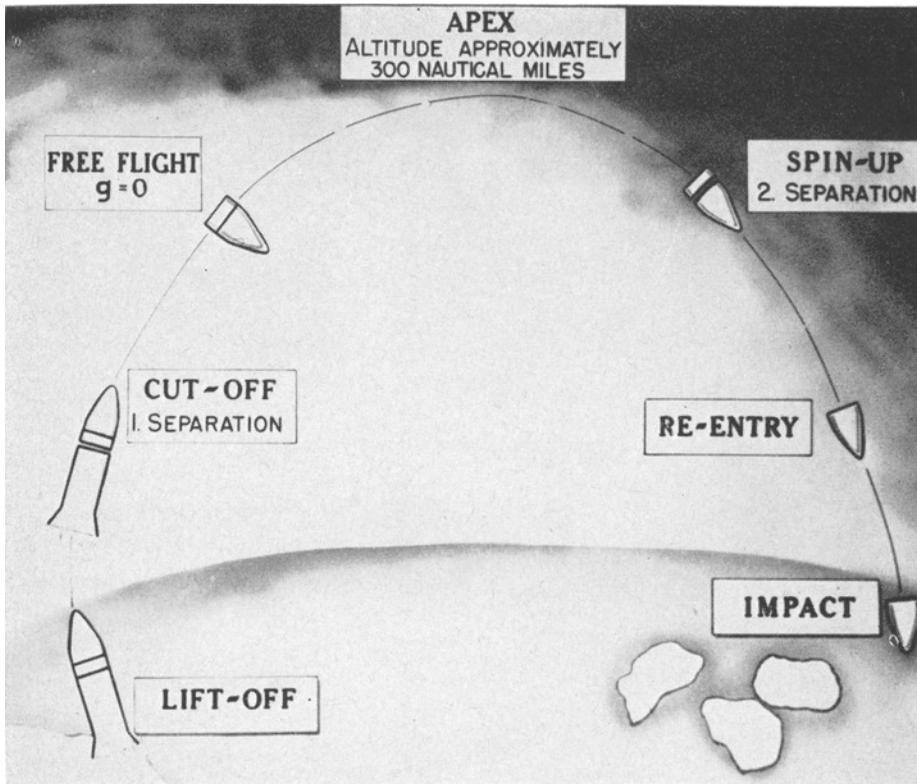
Fig. 1. Typical Jupiter trajectory. The curve describes the essential characteristics and main missile events of an IRBM flight.
