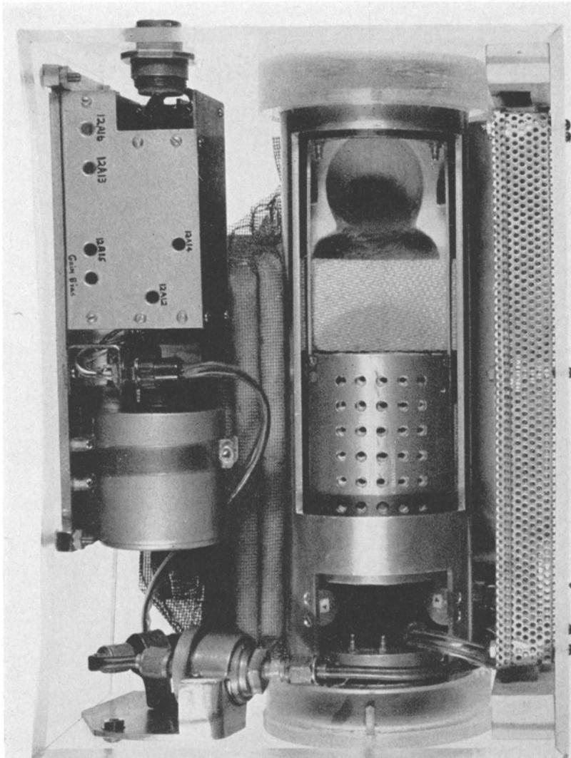
Fig. 4. Mockup of essential interior arrangements of Bio-Flight 1 capsule. The relative locations of the animal support system, the absorber tray, the absorber blanket, the electronic package, the oxygen pressure reducer and bleed valve assembly are shown. The oxygen supply bottle is located behind the absorber tray at the right.
