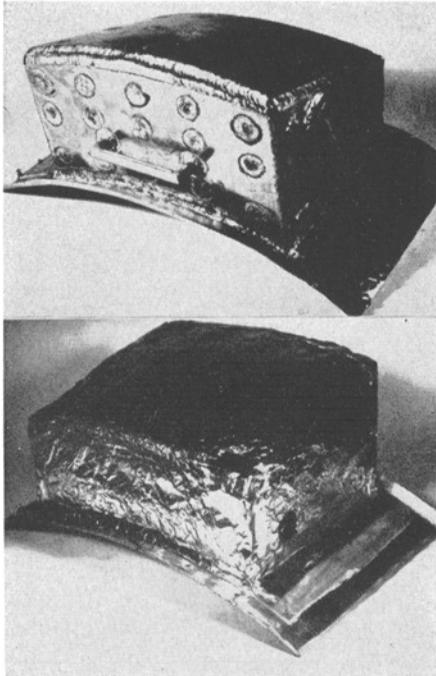
Fig. 2. Biocapsule for Bio-Flight 1. The upper photograph shows the capsule before, and the lower one after the final insulation coats have been applied.
