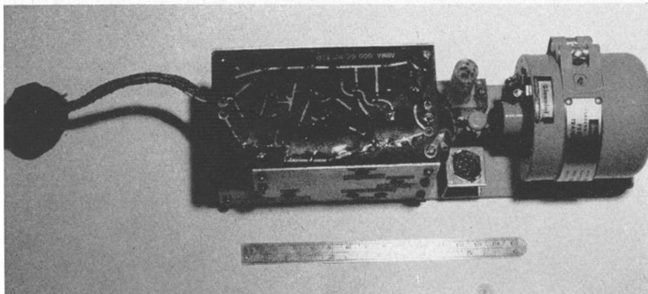
Fig. 5. Electronics package for Bio-Flight 1. The printed circuit amplifier boards, the ambient temperature and pressure transducers, and connectors are shown mounted on the base plate.
