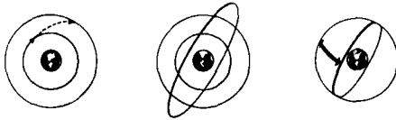
Fig. 2 Drawing showing the result of applying thrust in the space ship traveling in an orbit around the earth.
