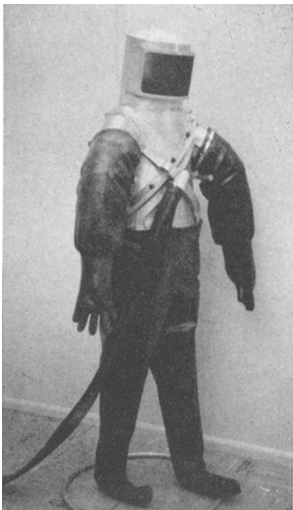
Fig. 2. Pressure suit with vapor cover, developed by Litton Industries, designed for use in experimental vacuum chamber.
