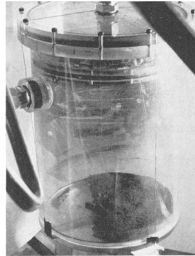
Fig. 4. Low temperature carbon collector after first filter blowback cycle.
